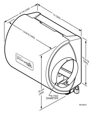
Fig. 2. Dimensions of HE265A,B in in. (mm).
